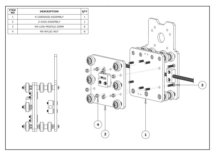
**A.** Mate the Z-Plate-Assembly to the X-Carriage-Assembly in the orientation seen above. Use 8 x M5-Low-Profile-20mm bolts and 8 x M5-Nyloc-Nuts to secure the two assemblies together. Make sure the Z-Plate-Assembly is square to the X-Carriage-Assembly. The allen key can be inserted through access holes on the X-Plate-Back to gain access to the bolt heads.
