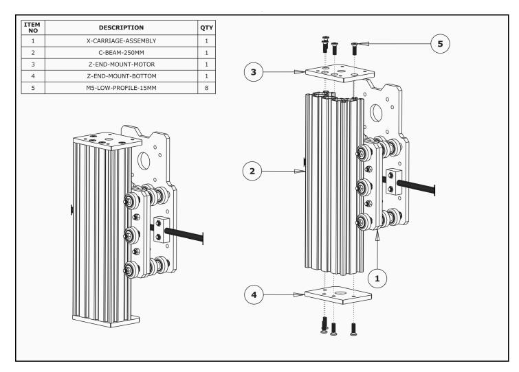
**A.** Slide the C-Beam-250mm through the Z-Wheels on the X-Carriage-Assembly. Attach the Z-End-Mount-Motor and Z-End-Mount-Bottom using 8 x M5-Low-Profile-15mm bolts. Tighten the Z-End-Mount-Motor bolts fully. For the Z-End-Mount-Bottom, tighten the bolts fully, and then loosen by a single full turn (the reason for this will become clear later).
