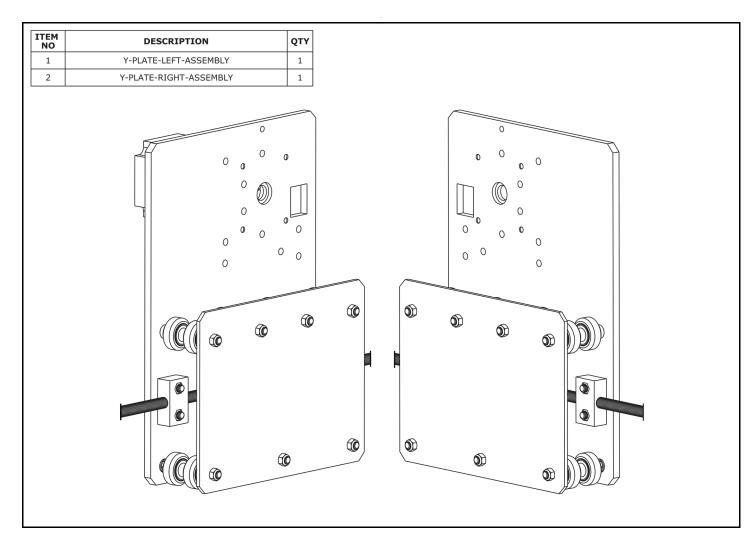
**A.** Except from Section 2.2.3, repeat the rest for Section 2.2 for the Y-Plate-Right. As seen above it should be a mirror image of the Y-Plate-Left-Assembly apart from the stepper motor.
